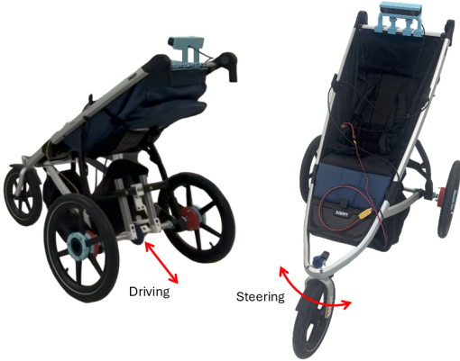
Figure 1: Overview of the stroller design with rear-wheel drive and front caster steering.
