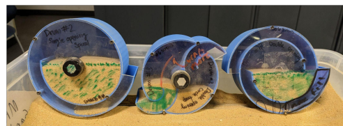
Figure 9: Subscale prototypes of potential bucket drum geometries with annotations after testing
